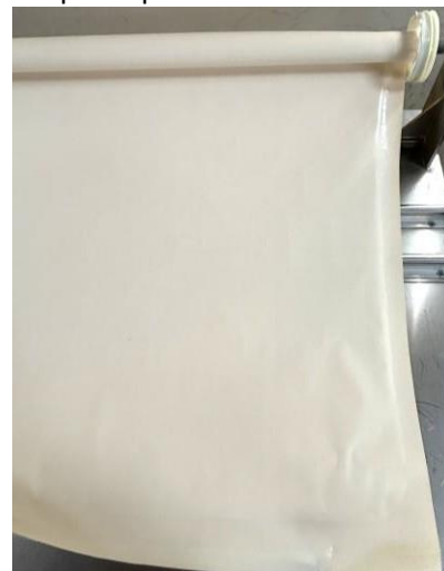
Photograph 20. Concentrate side of membrane leaf.
