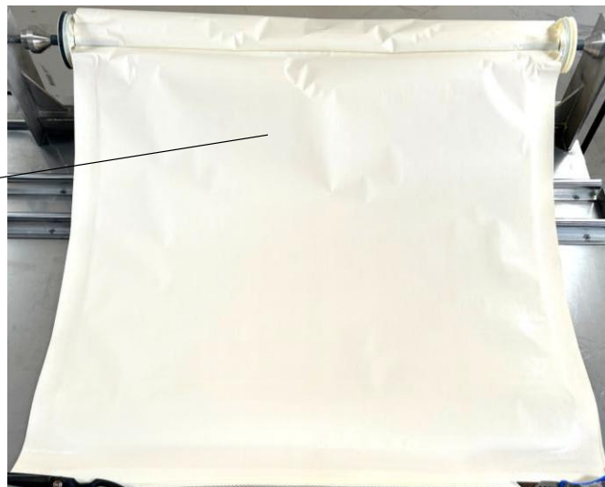
Photograph 13. Full membrane view of PA250601 (unrolled). Detail of spacer prints on the membrane surface.
