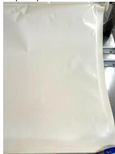
Photograph 15. Concentrate side of membrane leaf.
