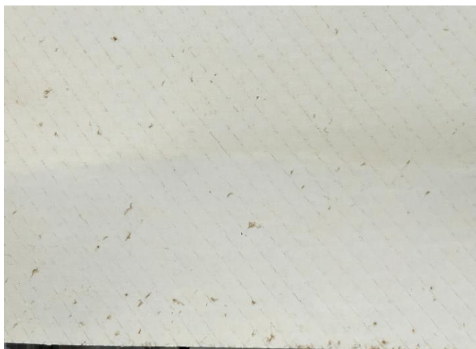
Photograph 23. Detail of membrane surface at feed end. Some dark particles are observed.
